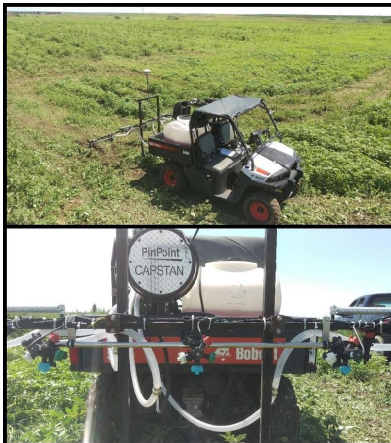
Figure 5.1. Capstan PinPoint® pulse-width modulation research sprayer at the 2016 Beaver City, Nebraska, field site.
