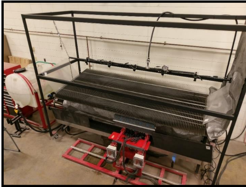
Figure 4.1. Spray patternator table with automated collection system used in this research located at the University of Nebraska-Lincoln in Lincoln, NE.
