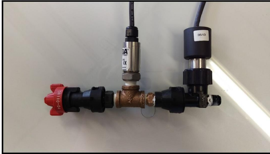
Figure 2.2. Nozzle body and pressure transducer assembly used to measure nozzle tip pressures after the pulse-width modulation solenoid valve. Another pressure transducer was connected inline 40-cm upstream from this assembly to provide gauge application pressure.
