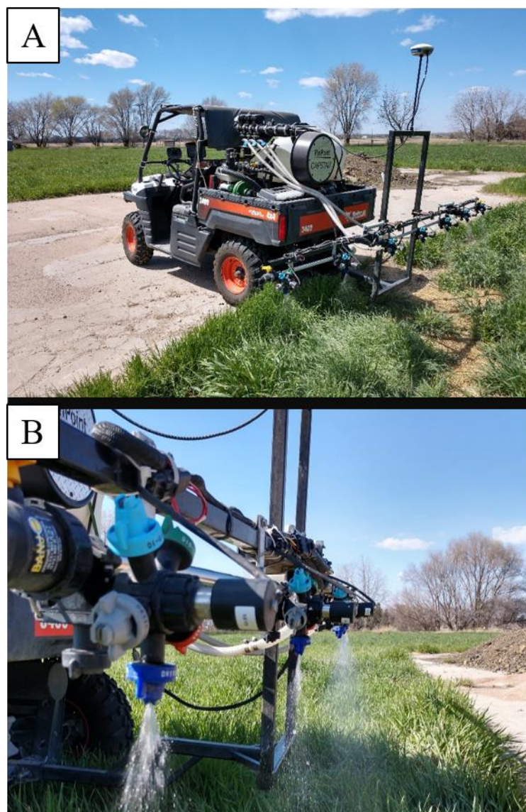
Figure 6.1. (A) Pulse-width modulation sprayer (Capstan PinPoint®) equipped and operated with (B) non-venturi nozzles (Wilger Industries Ltd., Lexington, TN, USA) used to apply droplet size treatments in this research.
