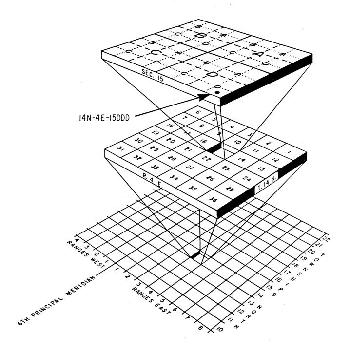
Fig. 1. System for identifying test-holes according to their location.
