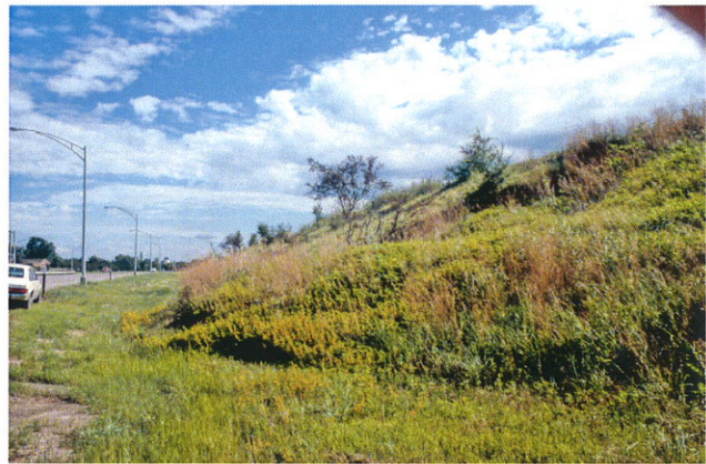
Fig. 51. Earth slump same site as Fig. 50. Quaternary System, Pleistocene loess underlain by glacial deposits. Tree in middle appears to be upright, while others were tilted.
