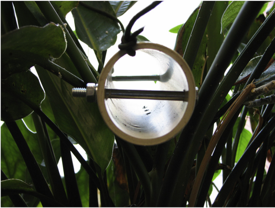
Fig. 3. Bait station (unbaited) to selectively deliver highly effective acetaminophen in a dead neonate mouse to brown tree snakes (Photo by P. Savarie).
