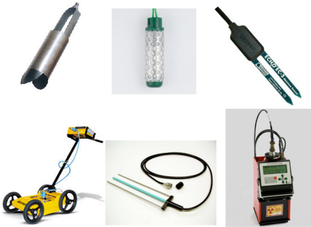
Fig. 3: Soil moisture sensors: Top row: Gravimetric, resistive (Watermark), capacitance, Bottom Row: GPR, TDR, neutron probe.
