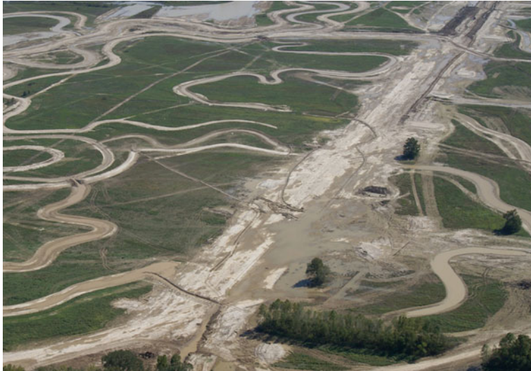
Fig. 3.12 Ditch filling and restoration of drainage pathways in Units A and B on the Duck Creek Conservation Area, Missouri
