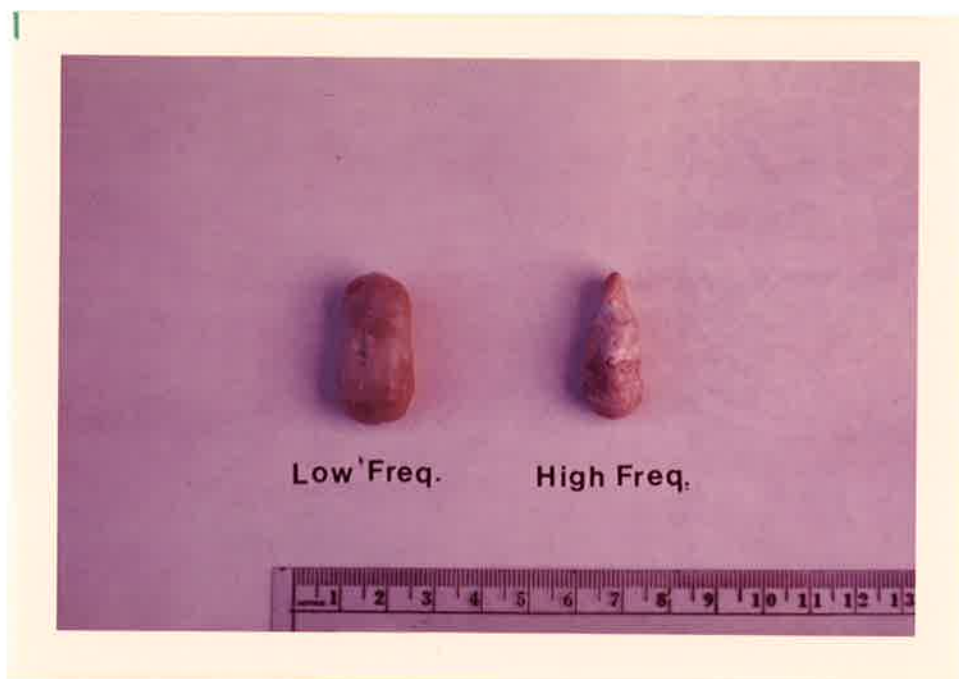
Figure 6, AVM SM1 Transmitter and Wildlife Materials Low Frequency Transmitter
