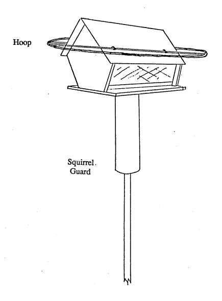
Fig. 3.2 Diagram of hopper with hoop treatment for pole-mounted hopper-type feeder.
