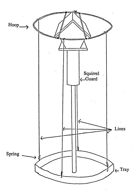
Fig. 1.1. Diagram of pole-mounted hopper-type feeder with hoop and lines.
