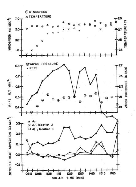
Fig. 15. Local (A<sub>1</sub>) and regional (A<sub>r</sub>) components of sensible heat advection over irrigated alfalfa at Mead, Nebraska (9 June 1976). Daily patterns of Rn+S, U (1.5 m, station 5), T (0.75 m, station 5), and e (0.75 m, station 5) are also shown.
