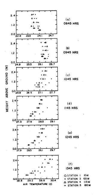
Fig. 8. Hourly temperature profiles (solar time) above irrigated alfalfa at Mead, Nebraska (10 June 1976) showing the transition from lapse to inverted profiles. Distances from the leading edge are indicated.
