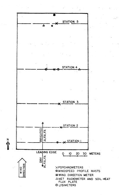
Fig. 4. Plan of the University of Nebraska Agricultural Meteorology experimental field (irrigated alfalfa), June-July, 1976.
