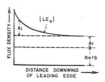
Fig. 2. Schematic of energy partitioning at the surface.
