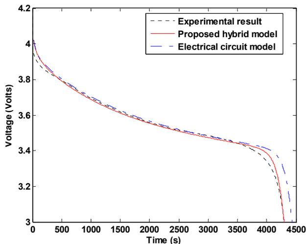
Fig. 8. Comparison of simulation results of the electrical circuit model and the hybrid model with experimental results for a single lithium-ion cell with a constant discharge current of 0.8C (2.06 A).
