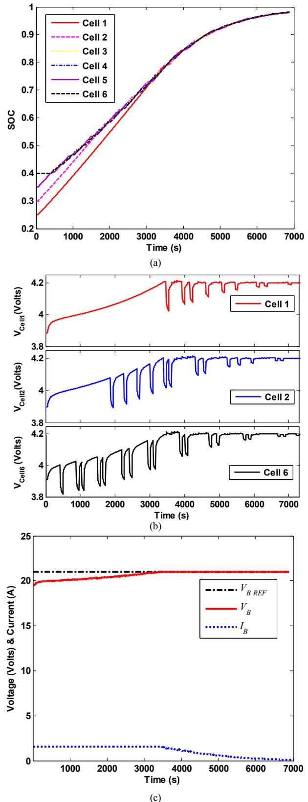
Fig. 10. Cell balancing control in the charge mode: (a) the SOC of each cell; (b) the terminal voltage of Cell 1, 2, and 6; (c) the terminal voltage and charge current of the battery.
