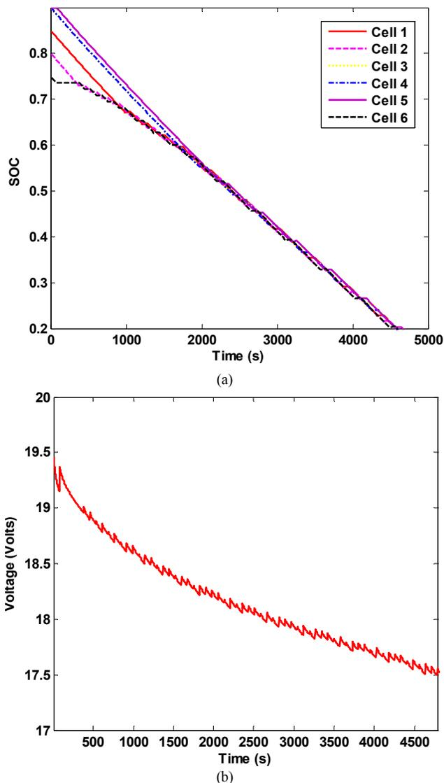
Fig. 11. Cell balancing control in the discharge mode: (a) the SOC of each cell; (b) the terminal voltage of the multicell battery.
