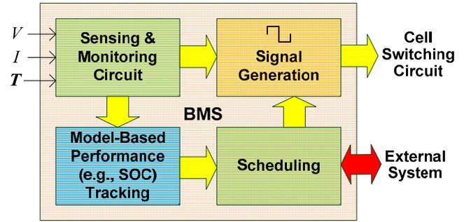
Fig. 5. The schematic of the battery management system (BMS).
