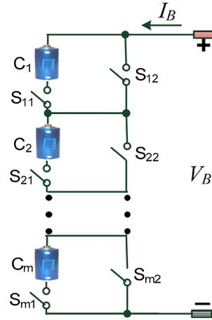
Fig. 2. The proposed series-connected, self-reconfigurable, multicell battery topology.
