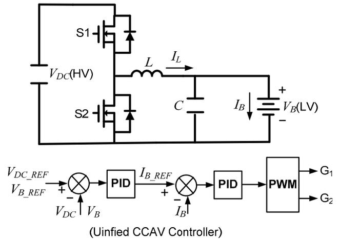
Fig. 3. The proposed bidirectional DC/DC converter with the unified CCAV controller for charging and discharging control of the multicell battery.
