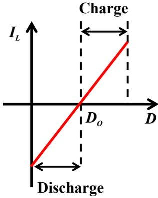
Fig. 4. Control duty cycle  $D$  versus average inductor current  $I_L$
