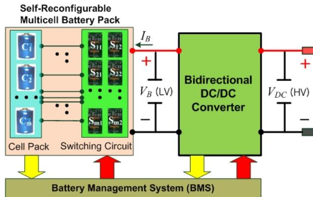
Fig. 1. The proposed self-reconfigurable multicell battery with a bidirectional DC/DC converter.
