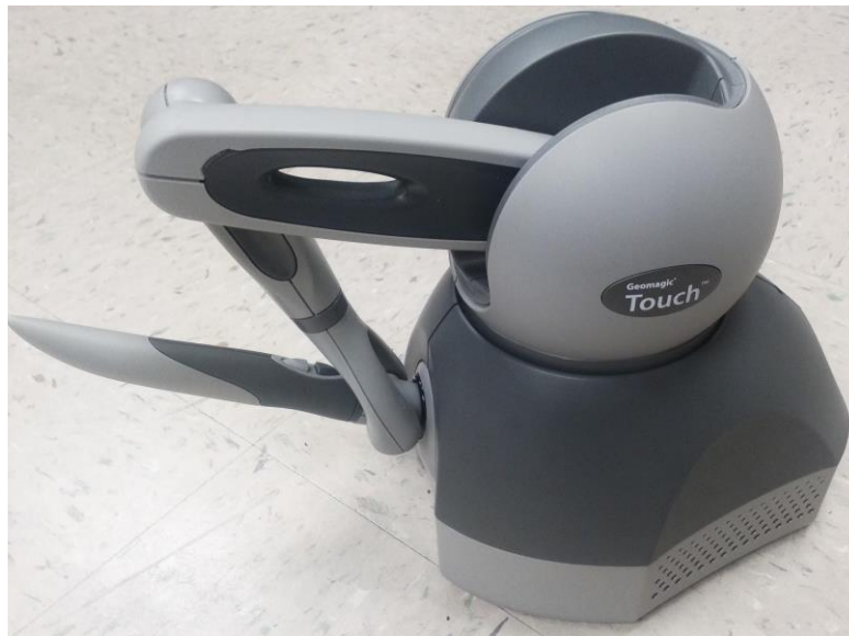
Figure 3.6 Geomagic Touch Haptic Controllers
