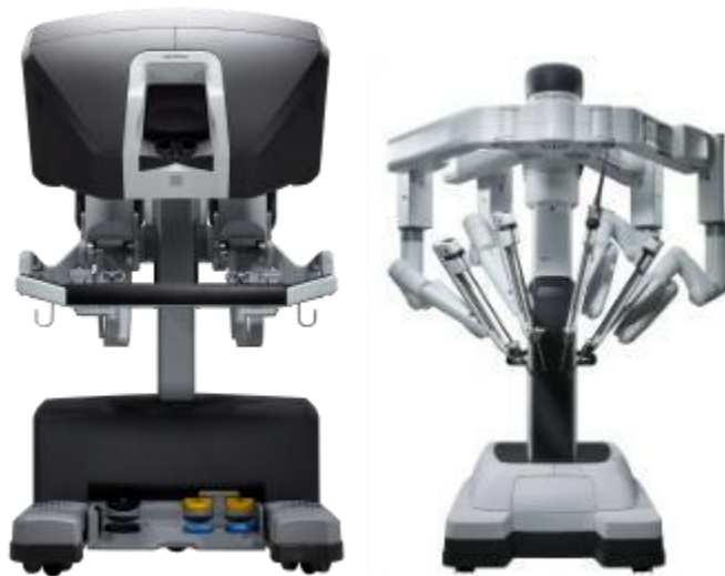
Figure 1.2 Da Vinci Surgical® System Control and Bedside Modules
