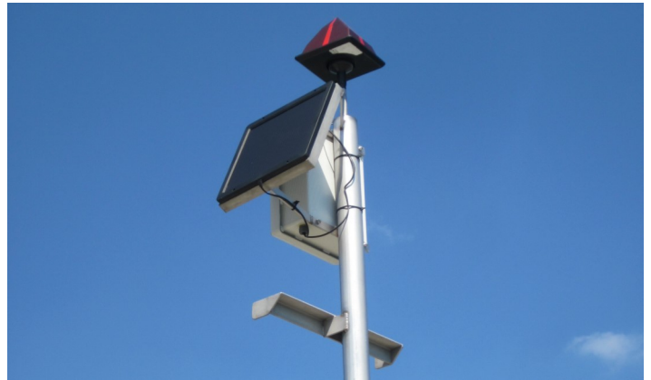
Figure 5. A solar-powered bird strobe sits atop a pole to deter bird use in an area.
