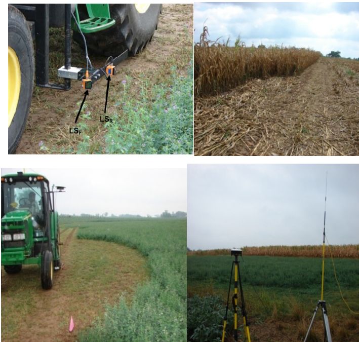
Figure 4. Sensor setup (top-left); Corn cut-crop edge (top-right); Sensor with RTK-rover vertically above the sensors (bottom-left); RTK-Base station (bottom-right)
