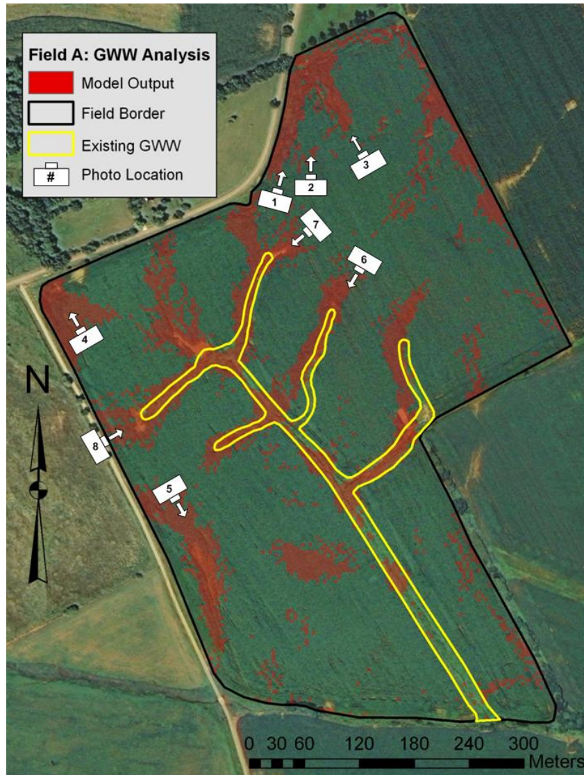
Figure 3. Aerial photograph of Field A identifying probability of erosion model output (values \geq 0.5 are shown in red), existing GWWs, and locations of photographed eroded areas.
