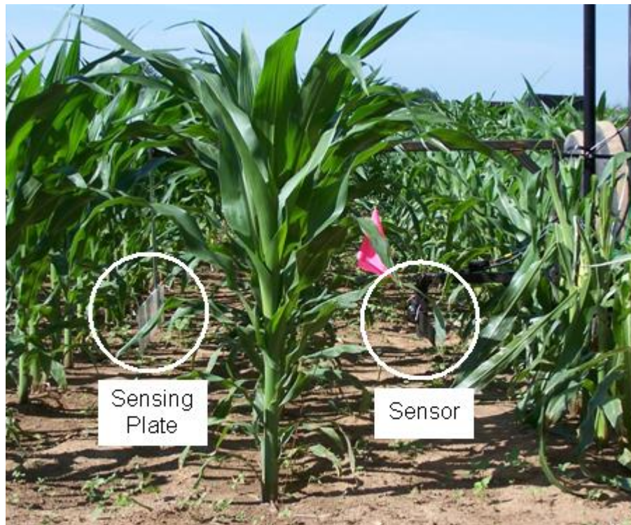
Figure 3. Field testing sensor placement with plate.
