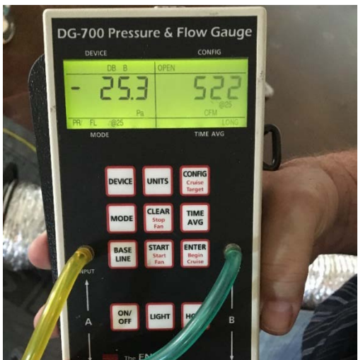
Figure 3.8 Duct Tightness Verification
