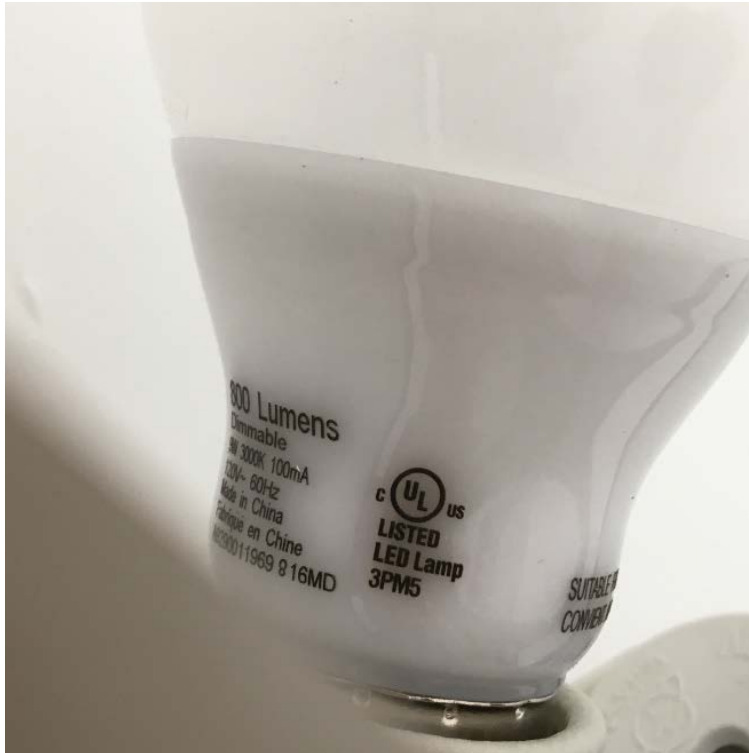
Figure 3.9 High Efficacy Lighting Verification
