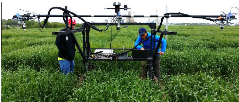
Fig. 1. The platform to mount the multi-sensor system for high throughput field phenotyping.
