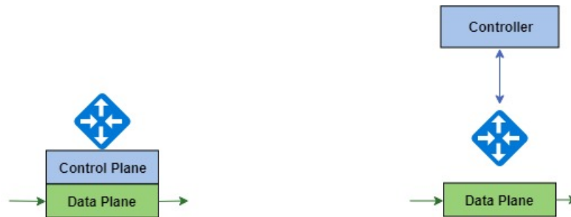
Figure 2.6: Traditional network vs Software-defined network
