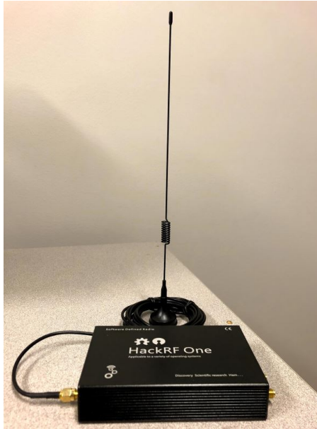
Figure 4.1: HackRF One— a low cost, open source software defined radio
