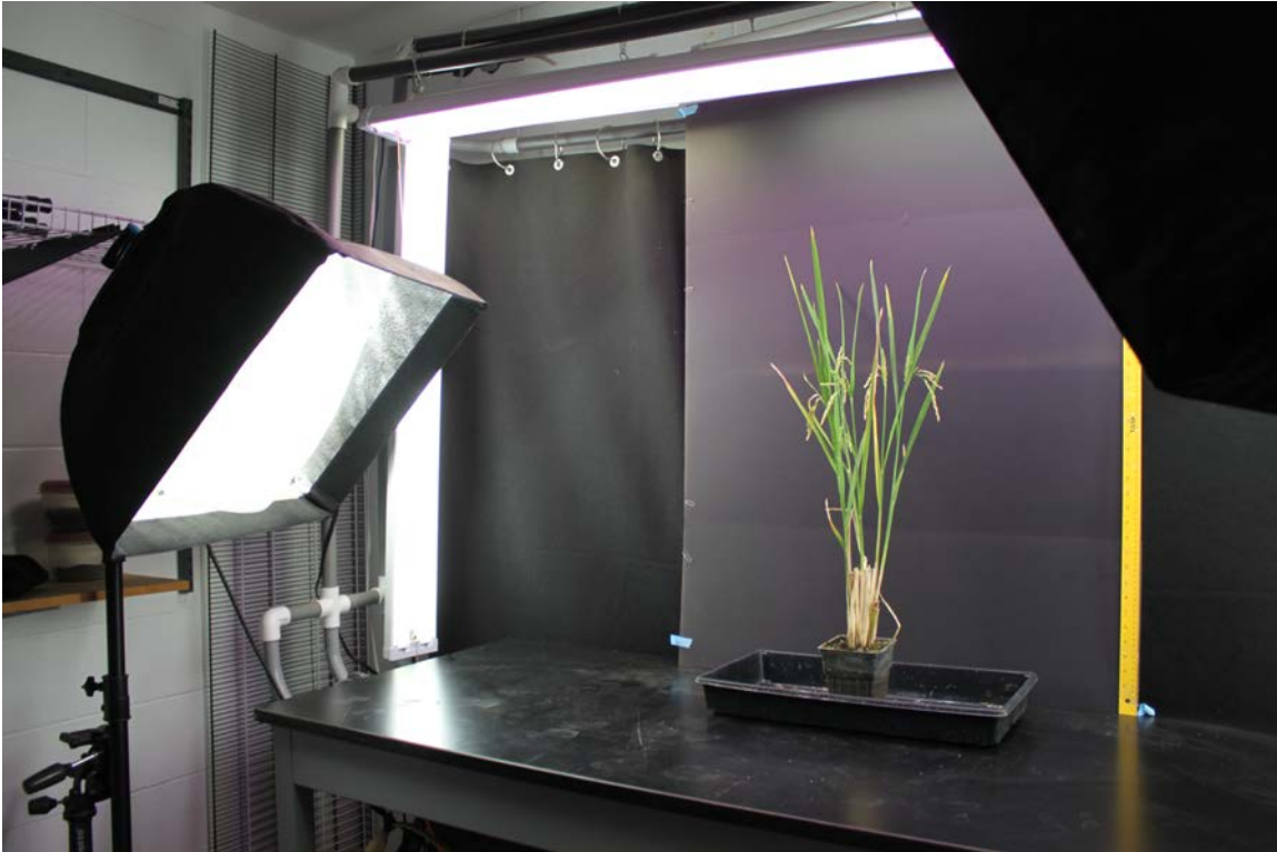
Figure S1. Imaging environment used for phenotyping with a conventional SLR camera. A imaging room was constructed to image a rice plant (cv 9311) at maturity in a homemade. To improve image processing several lighting sources were used to provide adequate light and a uniform background.
