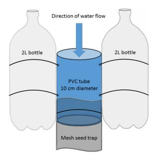
**Fig. 2** Floating aquatic traps used to characterize seed transport was characterized for 6 locations on the Platte River. The floating aquatic traps were designed to float half-way out of the water, so that material floating on the surface of the water was directed into a PVC tube (10 cm diameter) and collected in a mesh bag (triangular pores with a maximum width of 4.8 mm and length of 5.3 mm)
