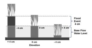
Fig. 3 The effects of flooding on seedling establishment were investigated in a controlled experiment conducted in rubberlined sections of greenhouse benches. Within a section cell, seedling flats were situated in one of three baseflow water levels: -4, 0, +4 cm. Flood treatments consisted of raising the water level 4 cm above the original elevation (0 cm) for different durations and at different times
