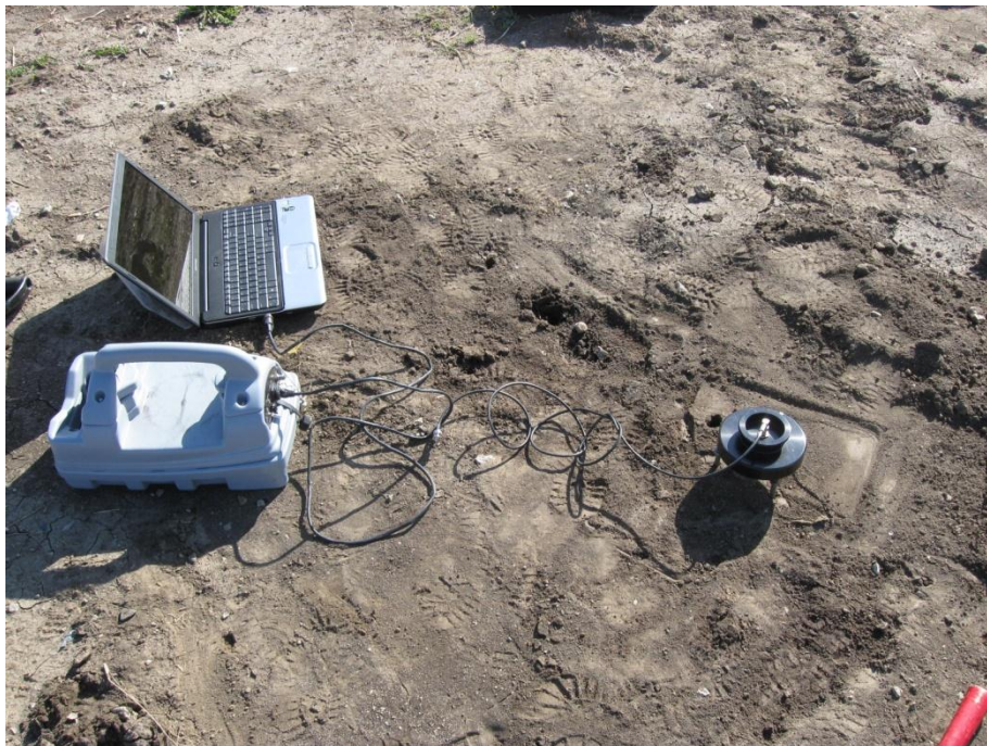
Figure 3.4. MDI connected to a laptop for density measurements
