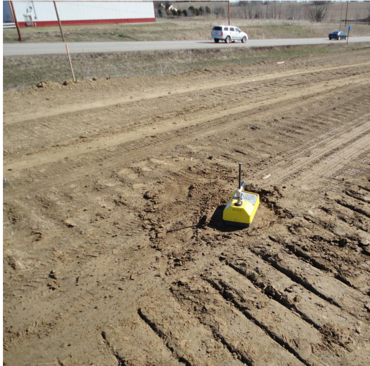
Figure 3.2. Nuclear gauge taking soil measurements
