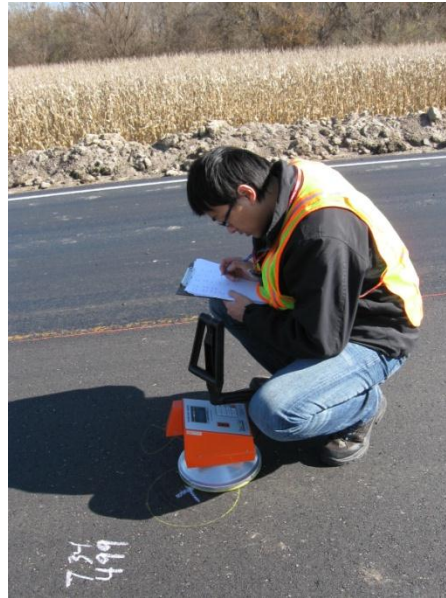
Figure 2.3. PQI model 301 shown taking measurements
