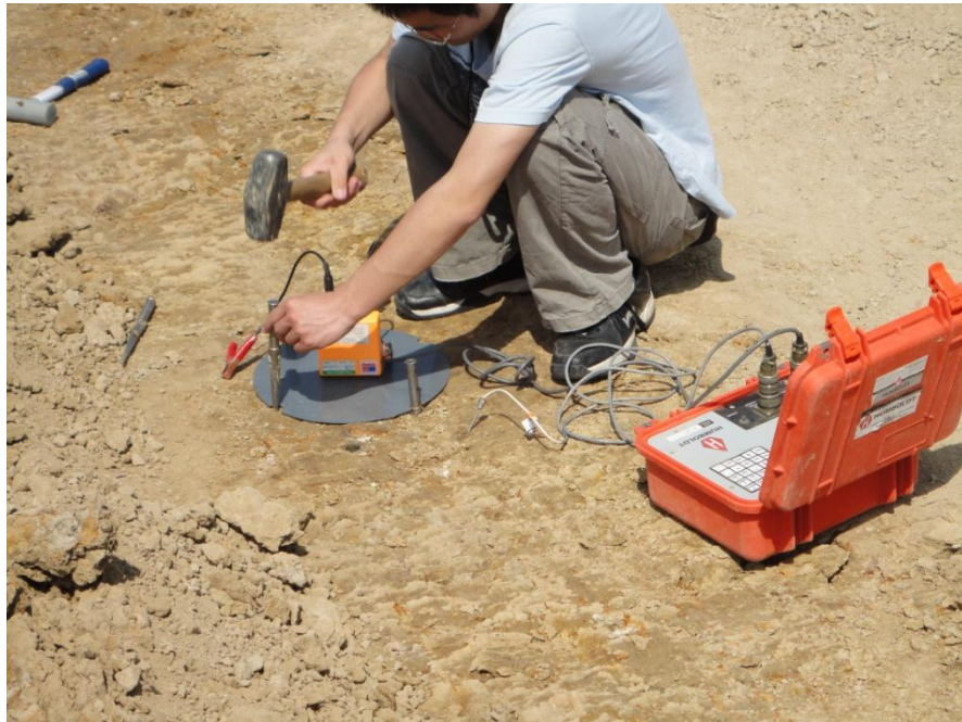
Figure 3.3. Darts driven into ground for EDG test
