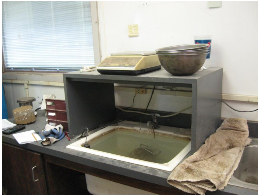
Figure 2.5. Lab set up for core measurements
