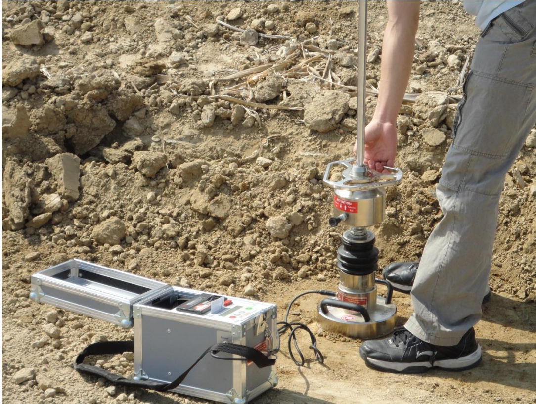
Figure 3.5. LWD is measuring stiffness of the soil
