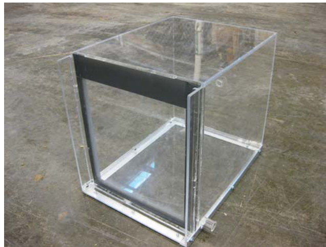
Figure 4. Box 2 anesthesia induction chamber (transfer chamber) with sliding door in place. Vapor ports are visible protruding from the side and on the rear of the chamber.
