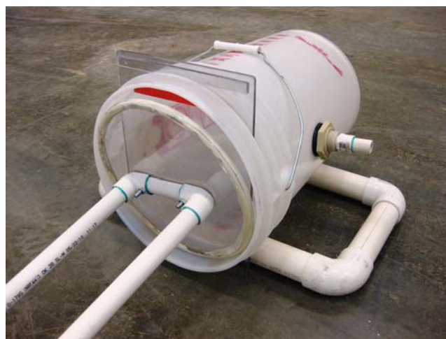
Figure 5. Cylinder anesthesia induction chamber with sliding door in place and plunger ready. Anesthesia hose attaches to the side-mounted vapor port shown.
