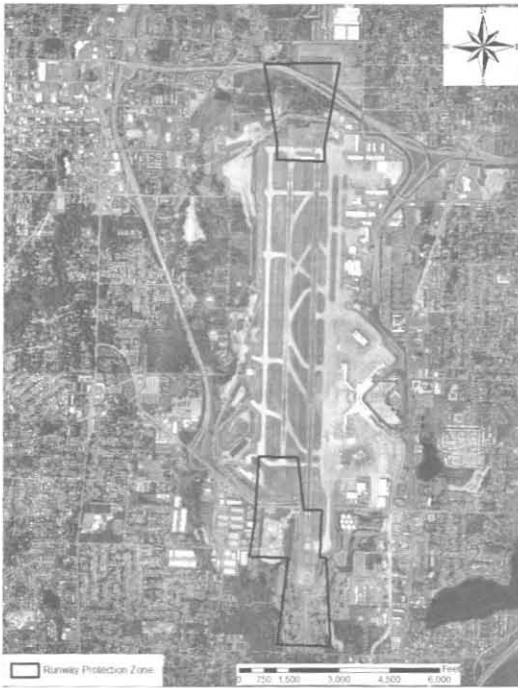
Fig. 14.2. Runway protection zones at Seattle-Tacoma International Airport, Seattle, Washington, USA. From Schafer et al. (2007)
