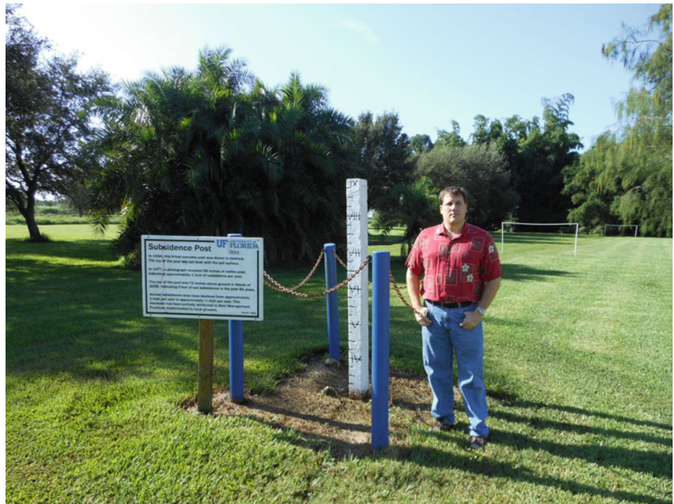
Fig. 18.5 Soil change through subsidence. This image shows the amount of subsidence that has occurred at the University of Florida's Everglades Research and Education Center, in Belle Glade, FL, since 1924 when a concrete post was driven into the organic soil so that it was level with the soil surface at the time. This photograph was taken in 2013 and represents about 1.8 m of soil loss. (Photograph credit: Alan Wright)
