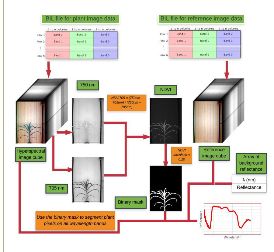
**Figure 5.** Steps in hyperspectral image processing
