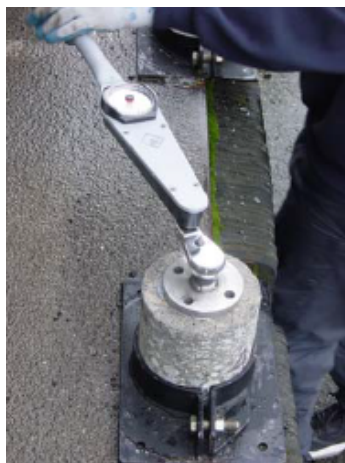
Figure 2-6. Torque bond test (Image from Tashman, 2006).
