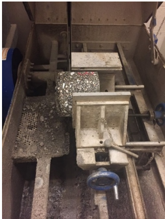
Figure 4-12. Cutting samples to prepare laboratory testing specimens.
