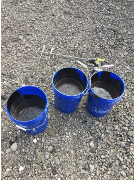
Figure 4-3. Dilution of emulsified asphalt.
