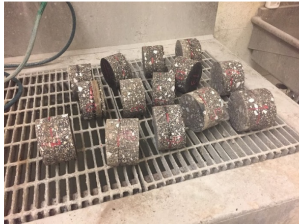
Figure 4-12. Cutting samples to prepare laboratory testing specimens.
