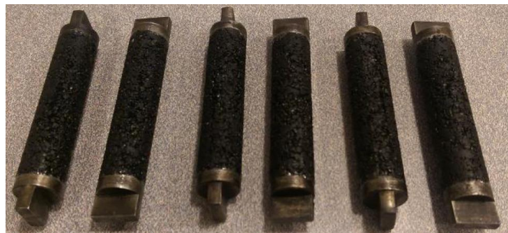
Figure 3-8. Fine aggregate matrix specimens with holders.
