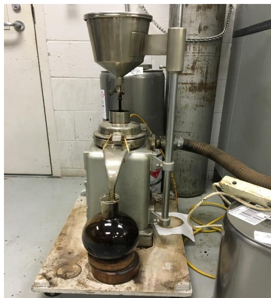
Figure 3-3. Micro-centrifugation of the solution after extraction.
