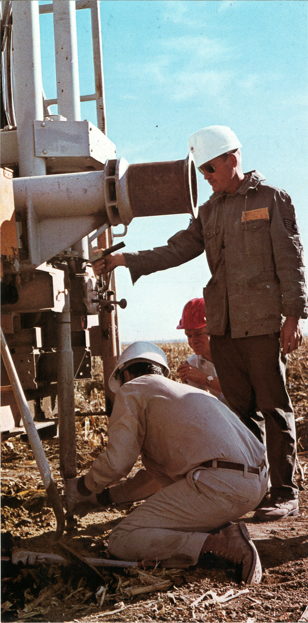
Left , near Seward, the drilling of a test hole, one of the state's 3,500. Photos by Jay Fussell.
