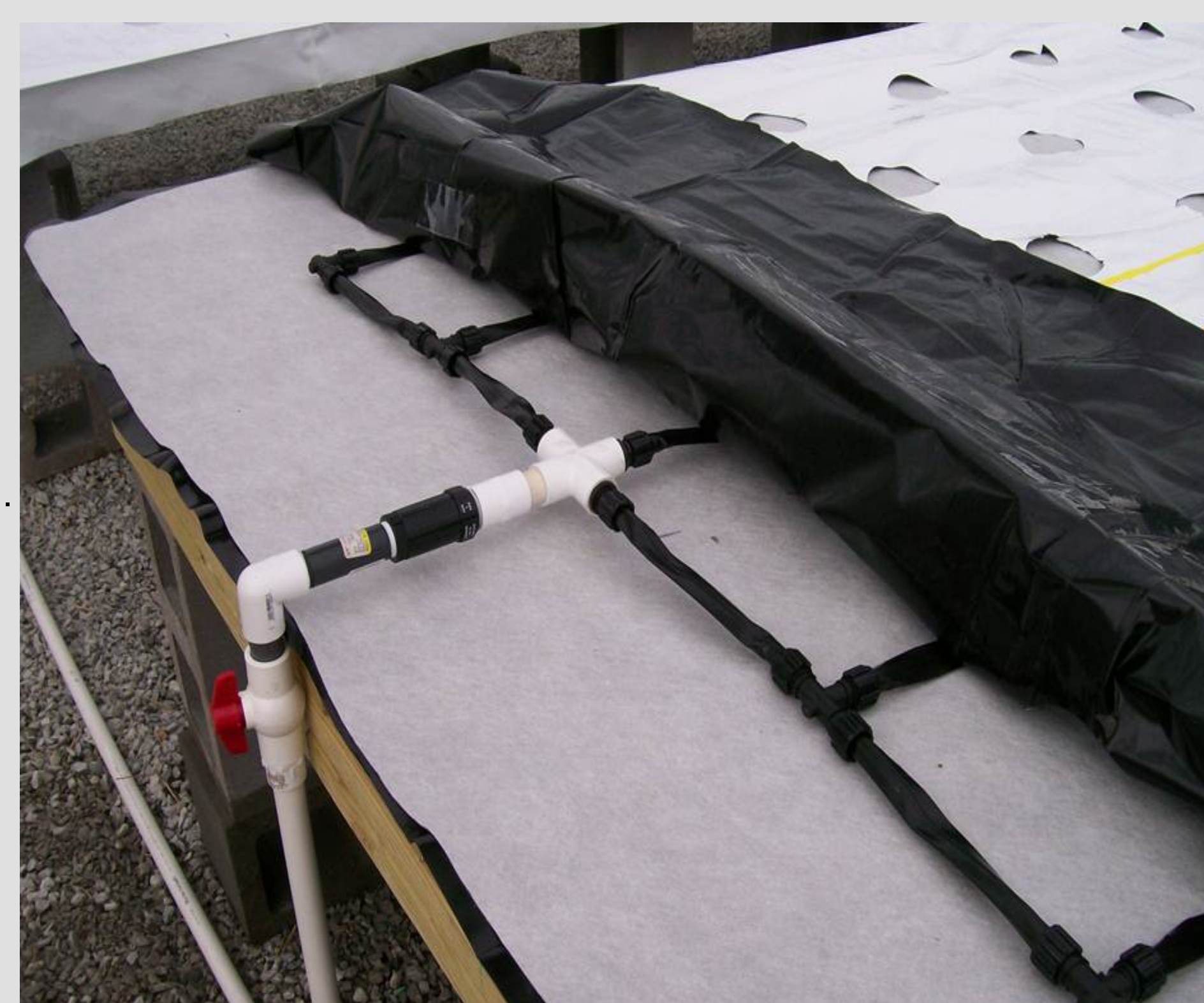
Figure 2. Capillary mat system with white/black polyethylene cover.
