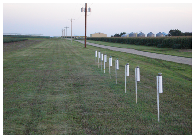
Figure 7. Evapotranspiration gages ( ET_{gage} ) with alfalfa and grass-reference canvas covers (#54 and #30, respectively) installed at the University of Nebraska-Lincoln, South Central Agricultural Laboratory (SCAL), Clay Center, Nebr., for research purposes. The research projects related to ET_{gage} and Watermark sensors conducted at SCAL are implemented into the NAWMDN functions.
