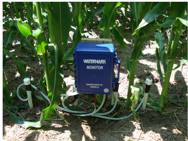
Figure 4. Watermark Monitor installed in a collaborator field to log the soil matric potential data on an hourly basis. Eight Watermark sensors can be attached to the monitor.
