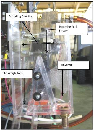
Figure  $\overline{3}$ . Flow diverter in the static weighing system of the flow meter calibration system at the Nebraska Tractor Test Lab.
