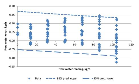
Figure 6. Flow meter errors and the 95% prediction band for the static weighing calibration (with No. 2 diesel fuel) of the Coriolis Effect fuel flow meter used during PTO dynamometer tests of tractors at the Nebraska Tractor Test Lab.
