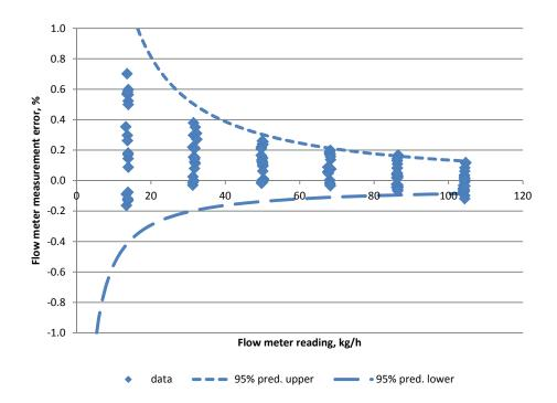
Figure 7. Flow meter errors and the 95% prediction band on a percent error basis for the static weighing calibration (with No. 2 diesel fuel) of the Coriolis Effect fuel flow meter used during PTO dynamometer tests of tractors at the Nebraska Tractor Test Lab.
