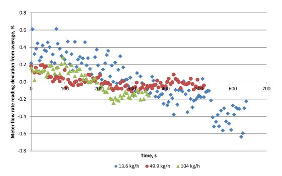
Figure 4. Meter flow rate reading deviations from average for the second replication of flow rate measurements using the dynamic weighing calibration method (with No. 2 diesel fuel) for the Coriolis Effect fuel flow meter used during PTO dynamometer tests of tractors at the Nebraska Tractor Test Lab.
