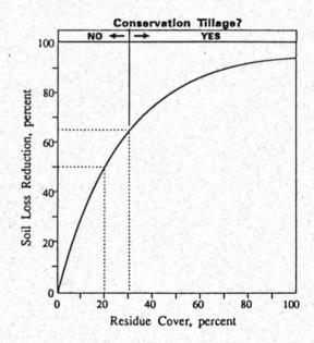
At least 30 percent of the soil surface must be covered with residue after tillage and planting is completed in order to be classified as conservation tillage. The examples show that a 20 percent residue cover will reduce erosion by about 50 percent of that occurring from a cleanly tilled field while a 30 percent cover can reduce erosion by as much as 65 percent.
