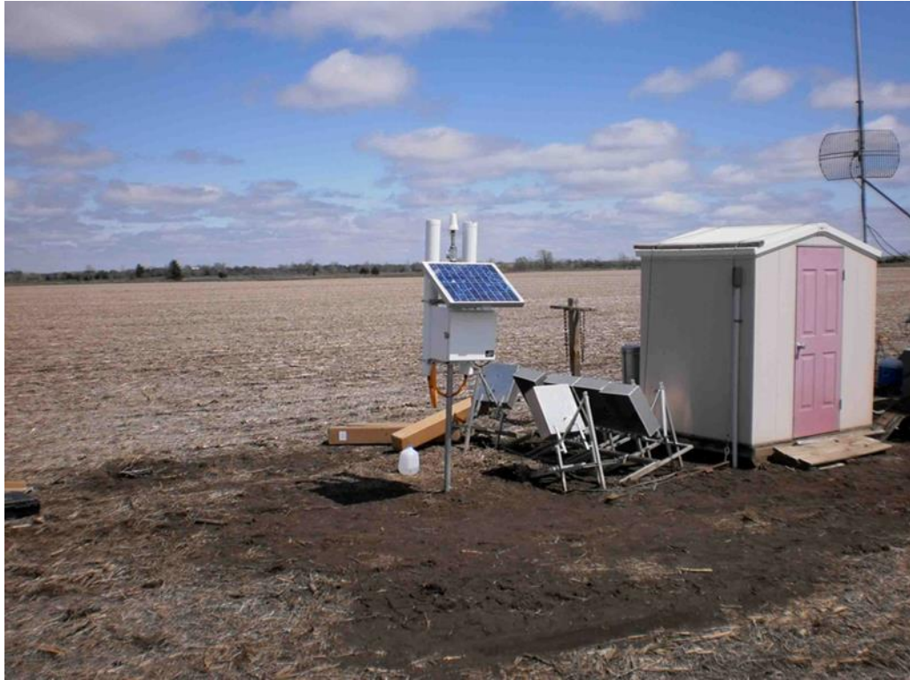
Figure 2.3: Cosmic-ray neutron probe at US-Ne3 site in Mead eastern Nebraska. The CRNP contains both bare and moderated detectors.
