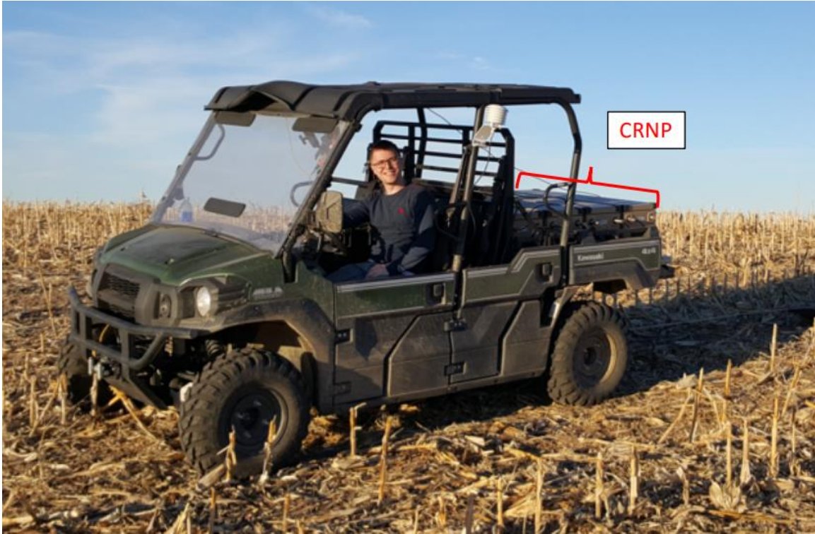
Figure 2.4: Mobile Cosmic-ray Neutron Probe Rover with moderated detectors only.
