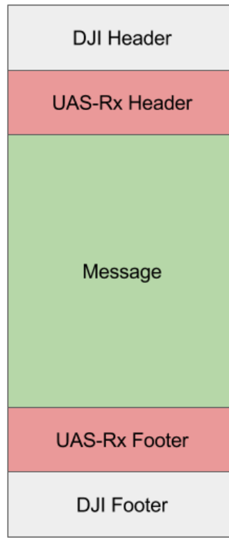
Figure 3.3: Protocol structure of a packet transmitted or received by the Dropper on the UART port.
