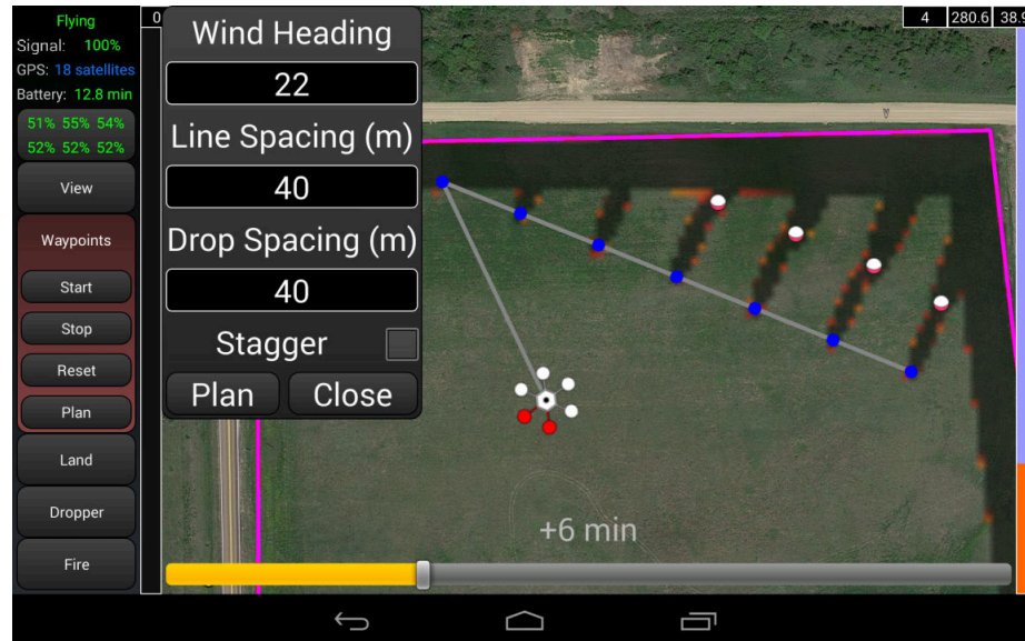
Figure 3.4: UAS-Rx Android application interface for planning ignition lines. The UAS-Rx is represented as a red and white hexacopter on the satellite map. A popup menu over the map has inputs for the ignition planner. The grey line and blue dots are the planned path and ignition locations. At the bottom is a yellow slider to project the fire simulation into the future. The slider is currently set at 6 minutes in the future, and the fire simulation shows how the planned ignitions would connect to the previous ignitions.
