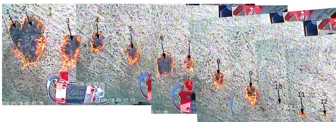
Figure 2.17: Video frames from a flyover of the ignition spheres dropped during the fifth flight at Homestead National Monument. Arrows point to locations ignition spheres were dropped.
