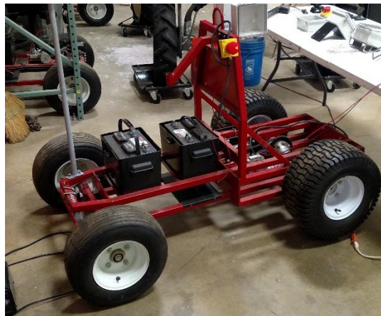
Figure 5.4 - Robot chassis including batteries, motors, and emergency-stop switches
