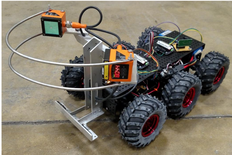
Figure 2.3 - Positioning and aiming of distance sensors behind leaf guard
