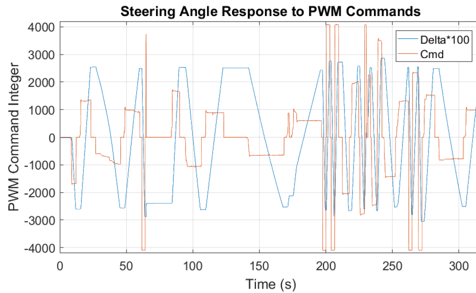
Figure 5.19 - Steering speed was linearly coupled to the PWM commands
