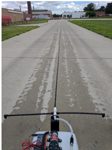
Figure 7.24 - Spray pattern from straight line navigation control
