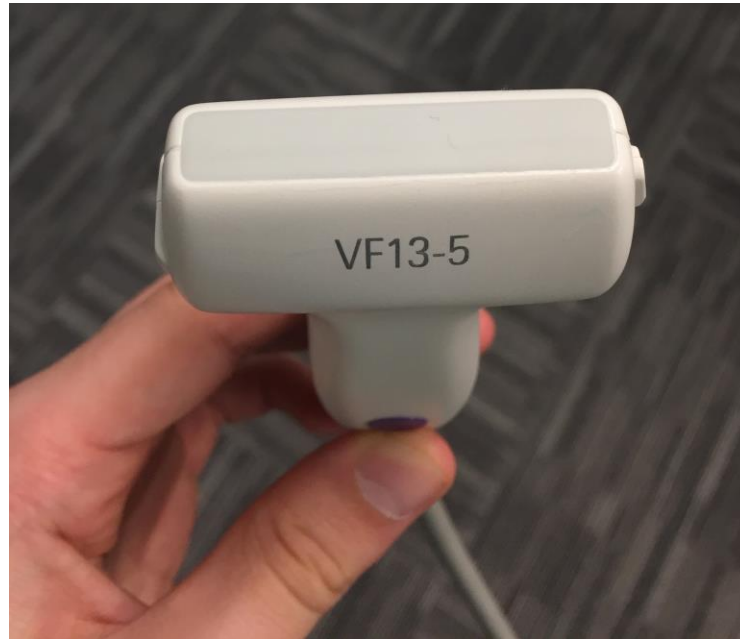
Figure 2.5 Typical ultrasound transducer used in medical imaging. The light gray band on the face of the transducer houses the components which transduce electrical energy into mechanical energy, and vice versa, to emit ultrasound into the body and record ultrasound echoes returning to the transducer.
