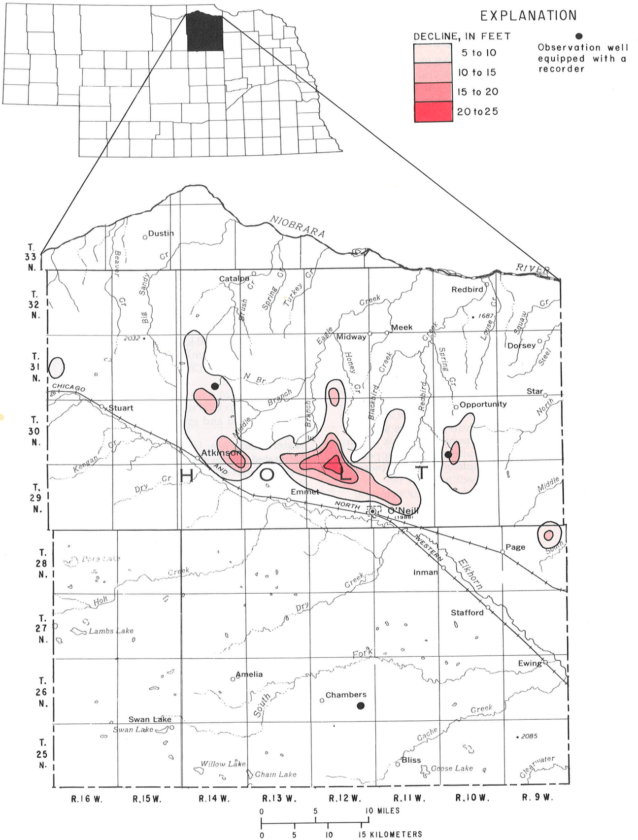
Areas of significant water-level change in the O'Neill area, from 1957 to fall 1977
