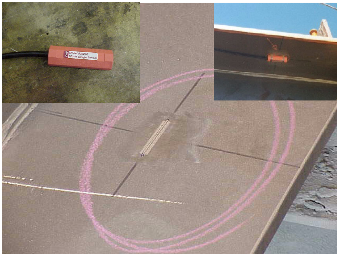
Figure 3-33: Steel strain gage and reader. Clockwise from upper left: reader, gage and reader in place, gage after being placed on reader.
