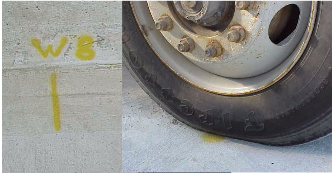
Figure C-1: Example of location to take measurement marked on deck (left) and front truck tire stopped at a location (right)
