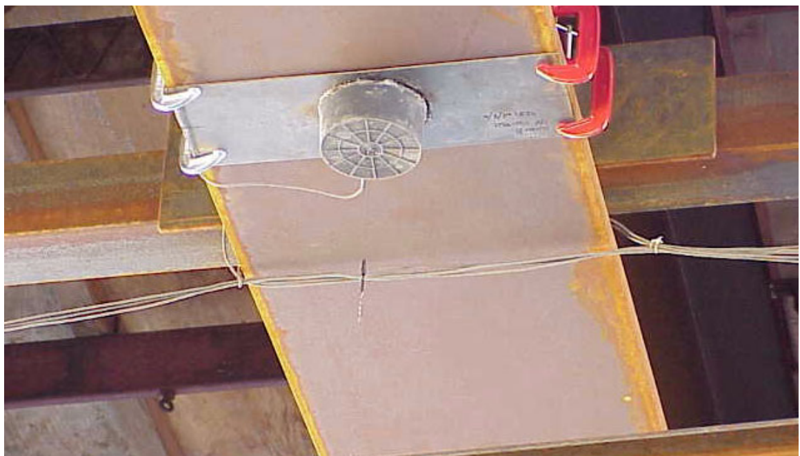
Figure 3-36: Potentiometer connected to the girder and fixed frame.
