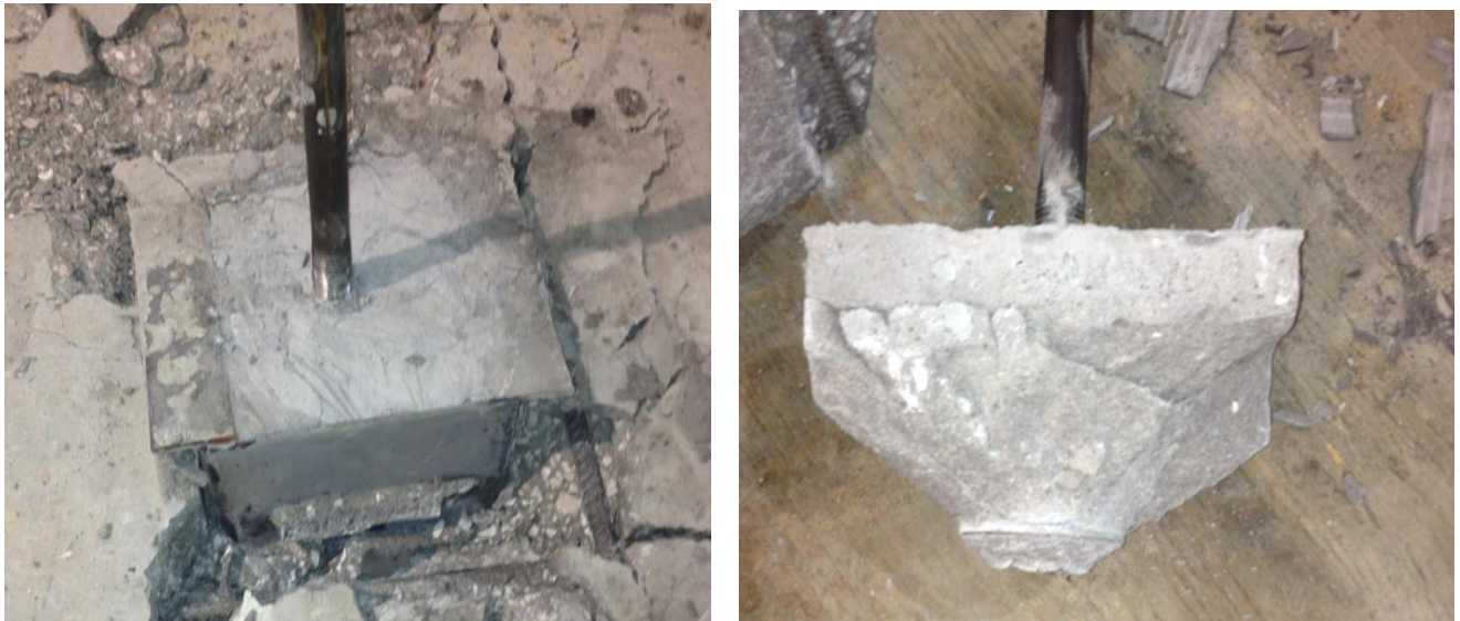
Figure 5.30: Pullout failure mode of HSS-formed pocket (left) and shear-keyed pocket (right)
