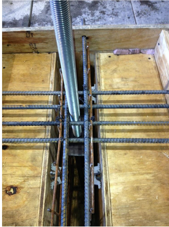
Figure 5.16: Deep T-girder specimen with anchor bars welded to the washer plate
