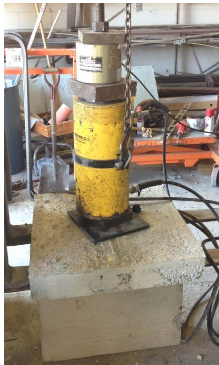
Figure 5.13: Pullout test setup of deep T-girder specimens
