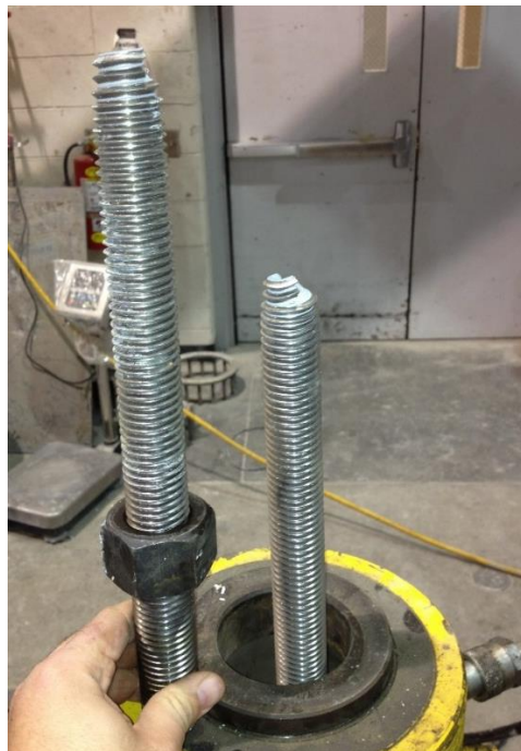
Figure 5.17: Rupture of the TR
