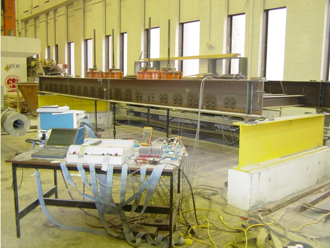
Figure 4-6. Two-Girder Bridge Ready for Loading and Data Acquisition System
