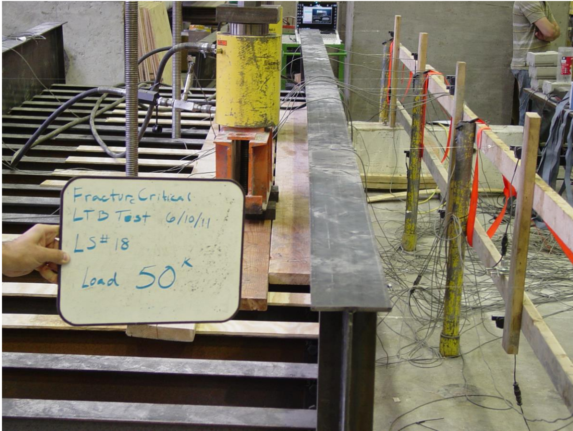
Figure 4-36. Deformed Bridge Under 50 kips of Load
