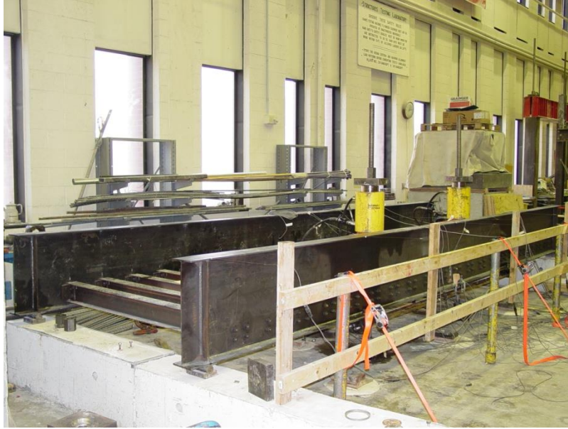
Figure 4-34. Test Bridge Setup Before Loading
