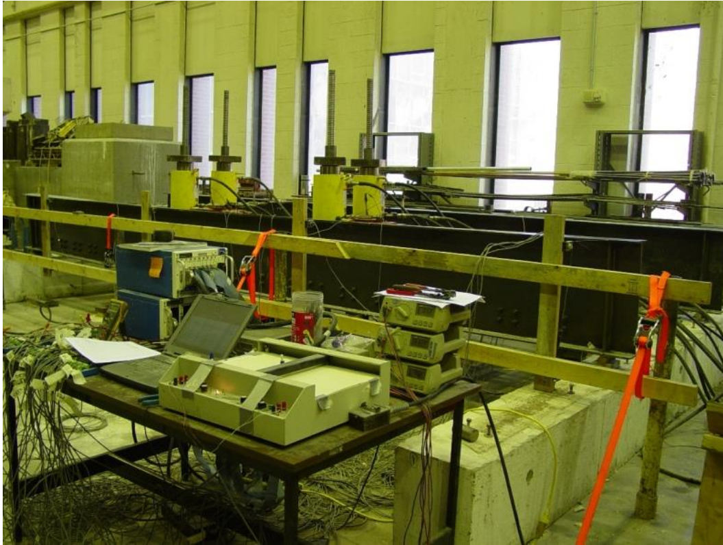
Figure 4-23. Data Acquisition and Test Bridge Setup (Initial Trial Loading Configuration)
