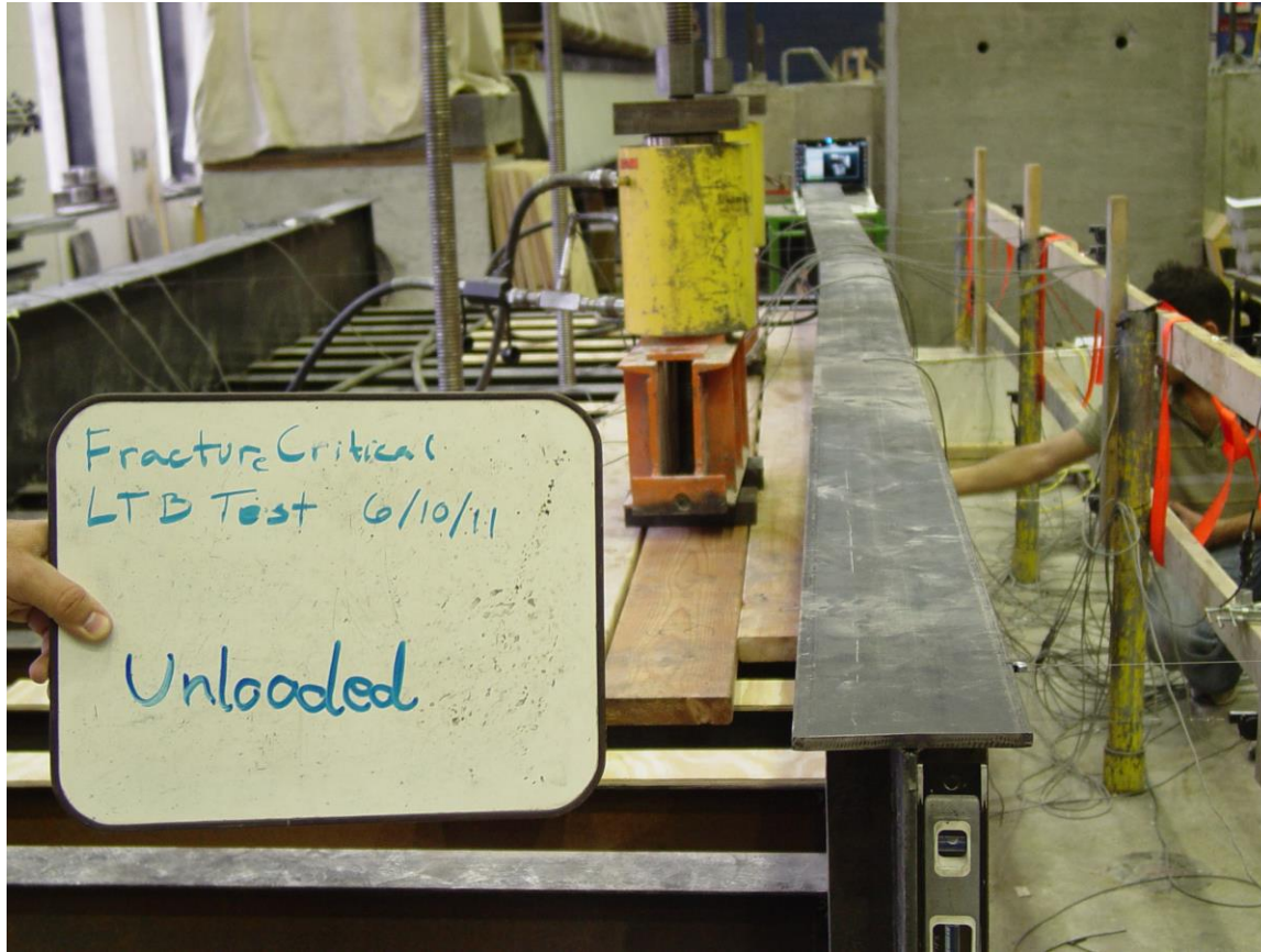
Figure 4-46. Plastic Deformation of Bridge after Load Removal
