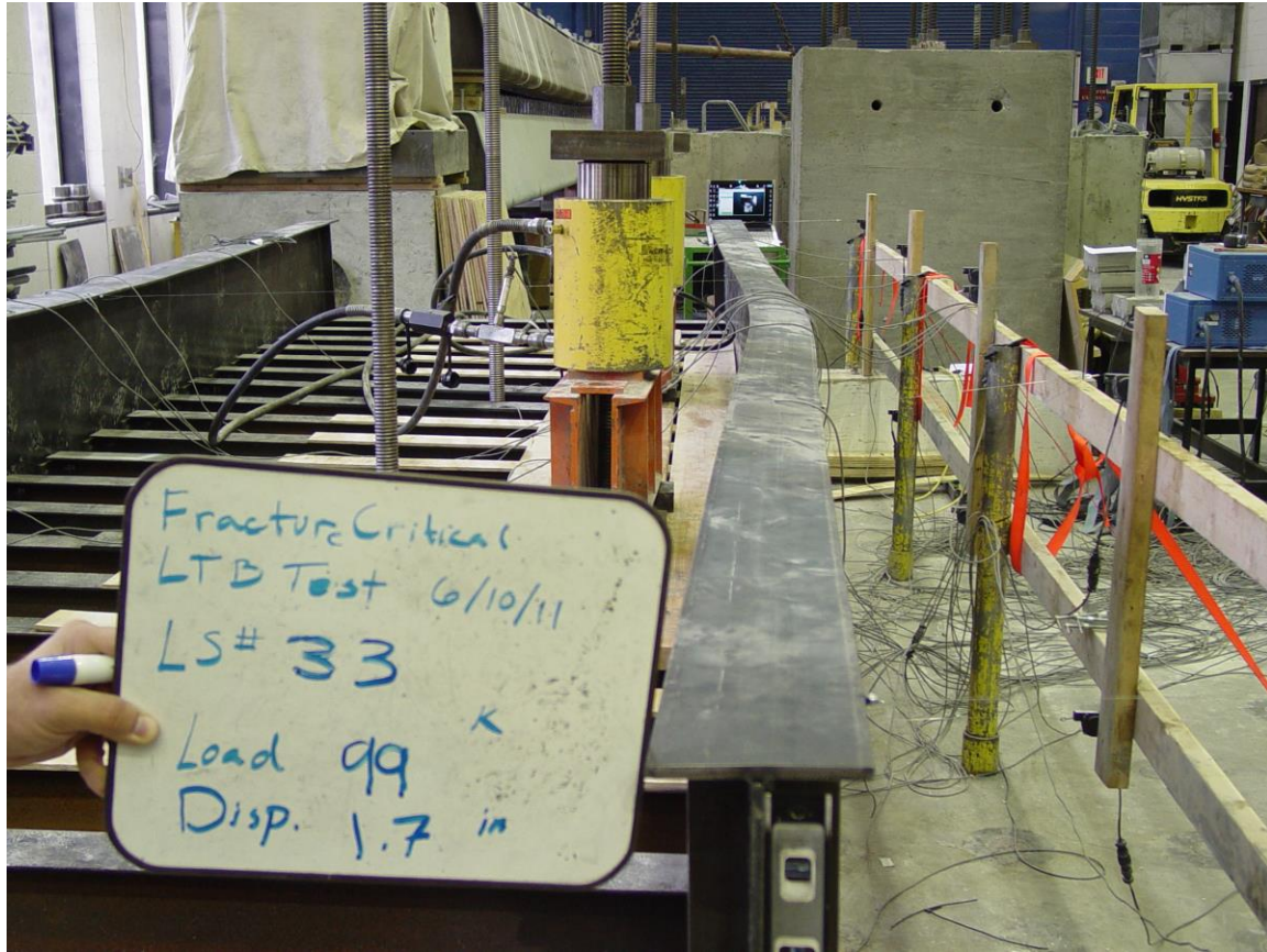
Figure 4-45. Deformed Bridge Under 99 kips of Load
