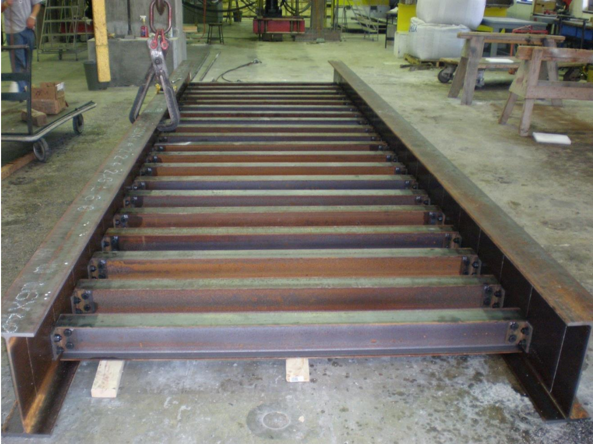
Figure 4-4. Assembled Two-Girder Bridge on Laboratory Floor
