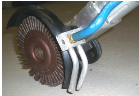
Figure 2.2 Behind wheel air nozzle
