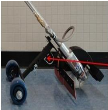
(a) 2 nd Generation : foldable wheel assembly
