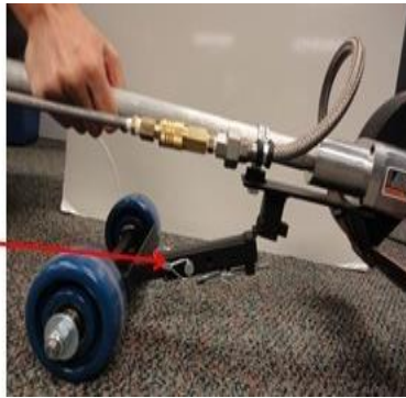
(a) 2 nd Generation : foldable wheel assembly
