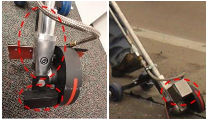
Figure 2.3 Pneumatically powered rotary motor & metal blocks
