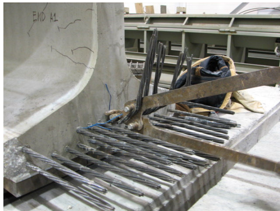
Figure 2.10.2: Second 45 degree strand bend
