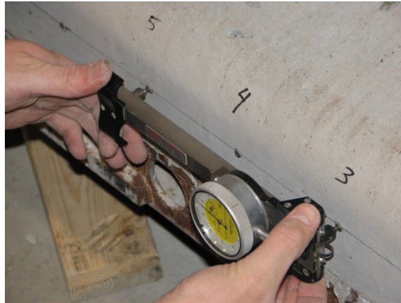
Figure 2.9.3: DEMEC point measurement
