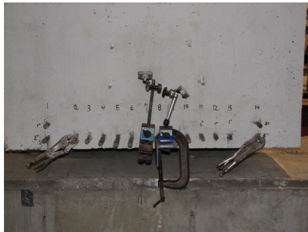
Figure 2.11.5.3: Caliper displacement gauges attached to the lower strands- end view
