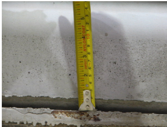
Figure 2.6.2: 5/8'' to 3/4'' initial camber
