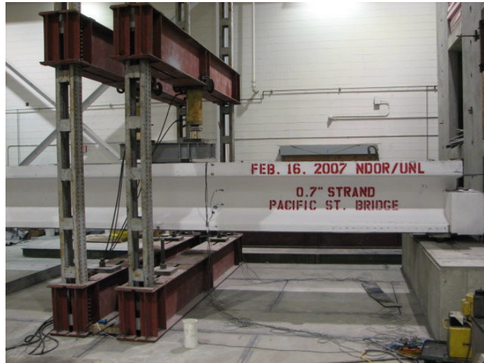
Figure 2.11.1.2: Girder test setup, double jacks and frames
