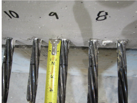
Figure 2.11.5.1: Strand slip measurement
