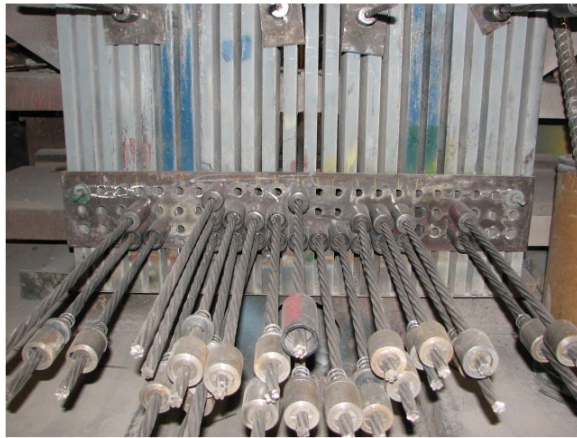
Figure 2.4.2.1: Jacking end pretensioned strands
