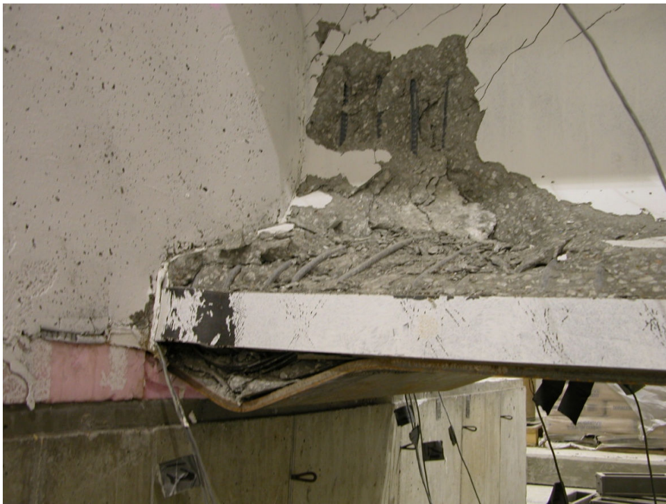
Figure 3.3.27: Specimen Failure at 382 kips
