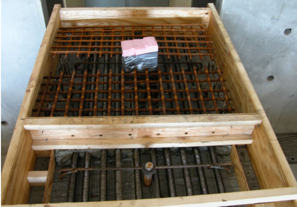
Figure 3.3.13: Reinforcement at the End Where Load Works On
