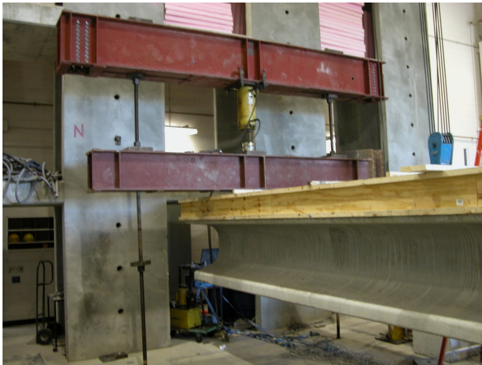
Figure 3.3.17: Deck, Girder and Diaphragm after Taking the Forms
