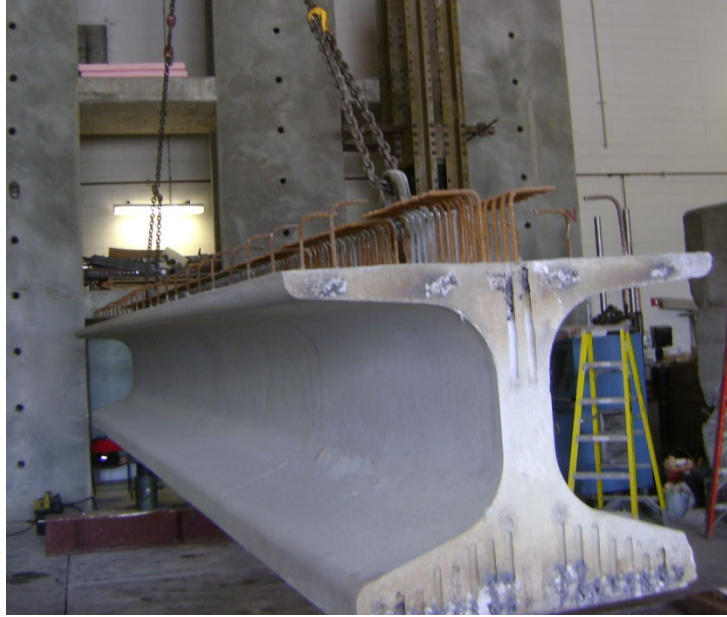
Figure 4.4.1: Placement of girder
