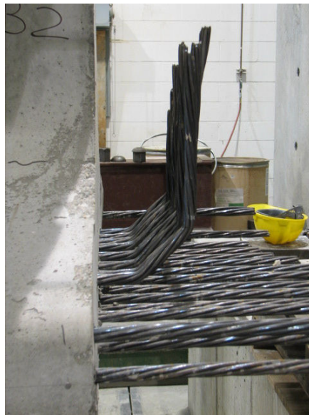
Figure 2.10.2: Second 45 degree strand bend
