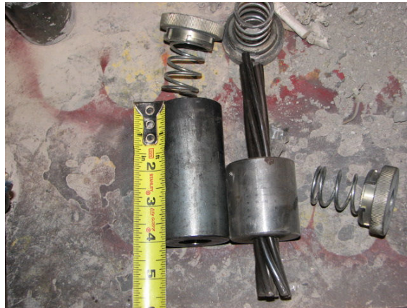
Figure 2.4.2.5: Reusable and one-time use chuck
