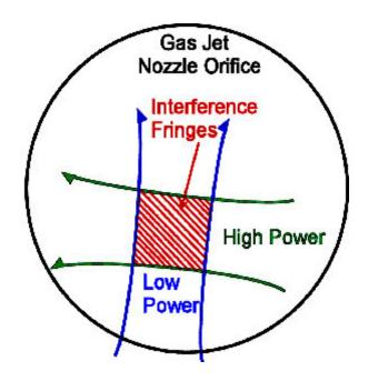
How does this effect come about? When the laser beams cross at right angles, an interference pattern forms. In the criss-cross zone (indicated by the bright light coming from the intersection region of the two beams in the photo), the interference pattern reflects light in much the same way as does a mirror, redirecting it perpendicular to its original travel. The interference also heats electrons.
