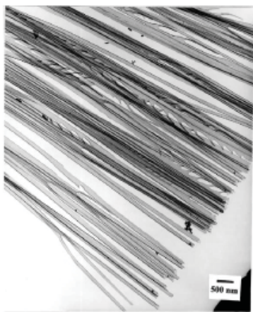
Fig. 4. TEM image of carbon tubes grown in PAAF anodized at 110 V.
