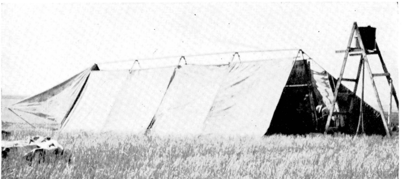
FIG. 2.—The application of water was protected from wind movements by a canvas cover.
