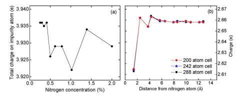
FIG. 3. (a) Charge on impurity atoms as a function on N-concentration; (b) Friedel charge oscillations: charge on the carbon atoms neighboring nitrogen impurity, as a function of distance from nitrogen atom.
