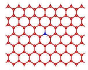
FIG. 1. Geometry of the N-doped graphene used in the calculations. Red indicates carbon, and blue indicates nitrogen.
