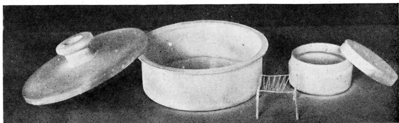
FIG. 3.—Relative humidity chambers, with accessories used in viability experiments.
