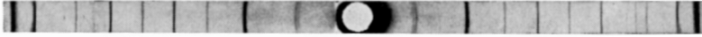
Fig. 43-11 X-ray powder diffraction pattern of tungsten obtained with a photographic film bent in the form of a circular cylinder. X-rays from a copper target were used in making this photograph. (From a photograph made by L. L. Wyman and supplied by A. W. Hull.)
