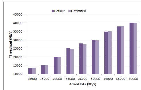
Figure 6.8: Comparison of actual throughput obtained in our experiments versus expected throughput
