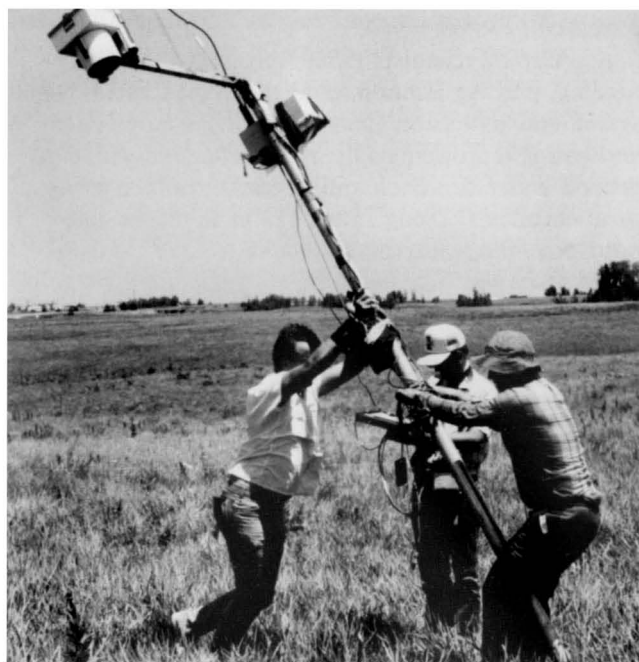
Instruments to measure radiation from prairie vegetation are used to duplicate data collected by satellites.
