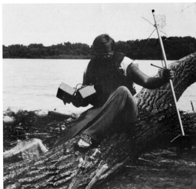
Locating a radio-tagged channel catfish in the Platte River using a hand-held antenna and receiver.
